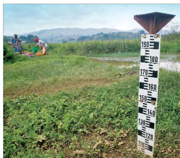
A post for measuring the tidal flows in the marshlands. Rugezi, Rwanda. FAO/Giulio Napolitano
