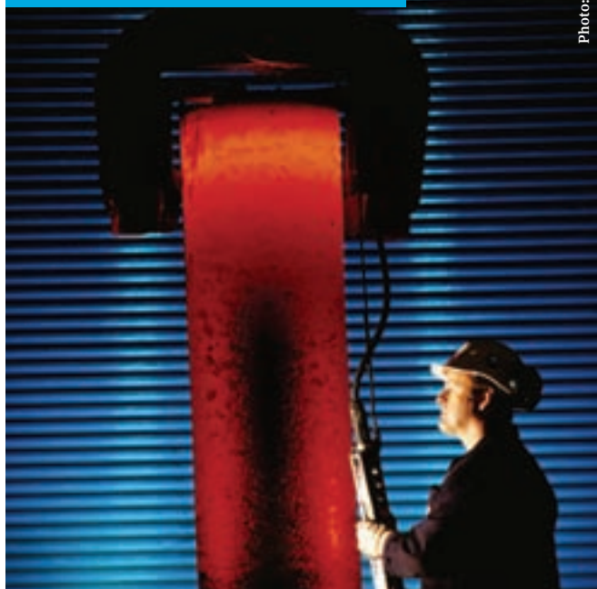
Vacuum Arc Remelted steel (VAR) for aerospace applications
